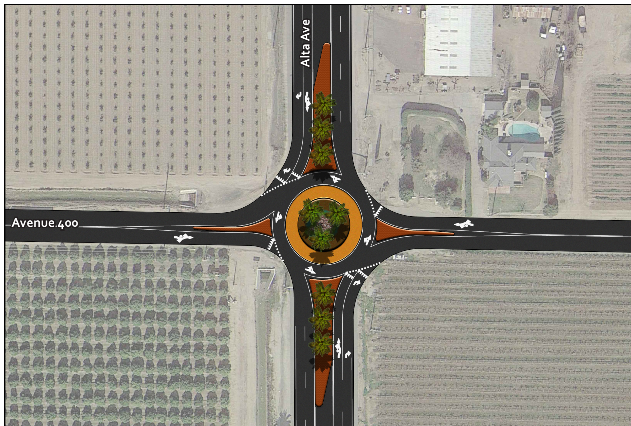
Figure 4-6. Proposed Design Concept for Alta Avenue & Avenue 400.
