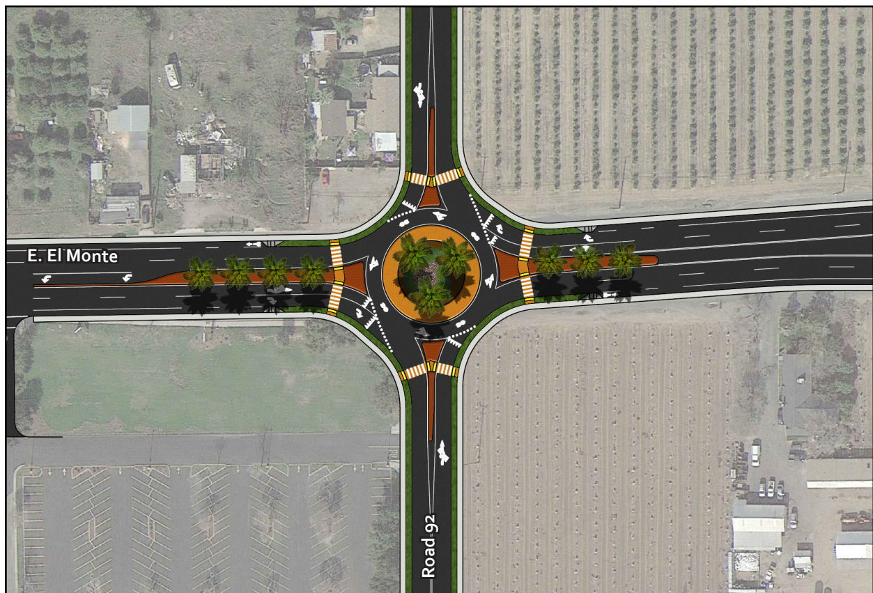
Figure 4-3. Proposed Design Concept for W. El Monte & Road 92.
