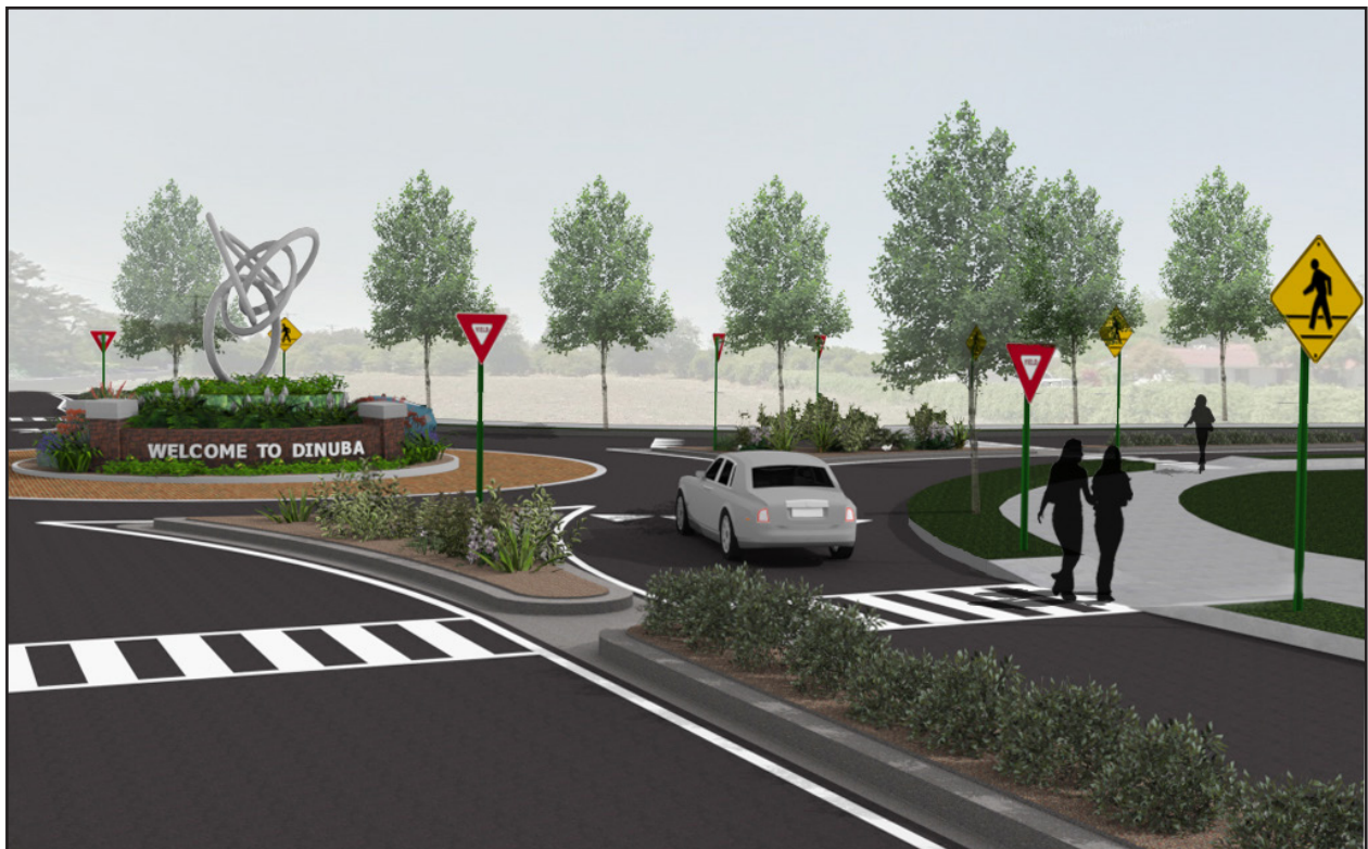
Figure 4-8. Conceptual splitter island landscaping.
