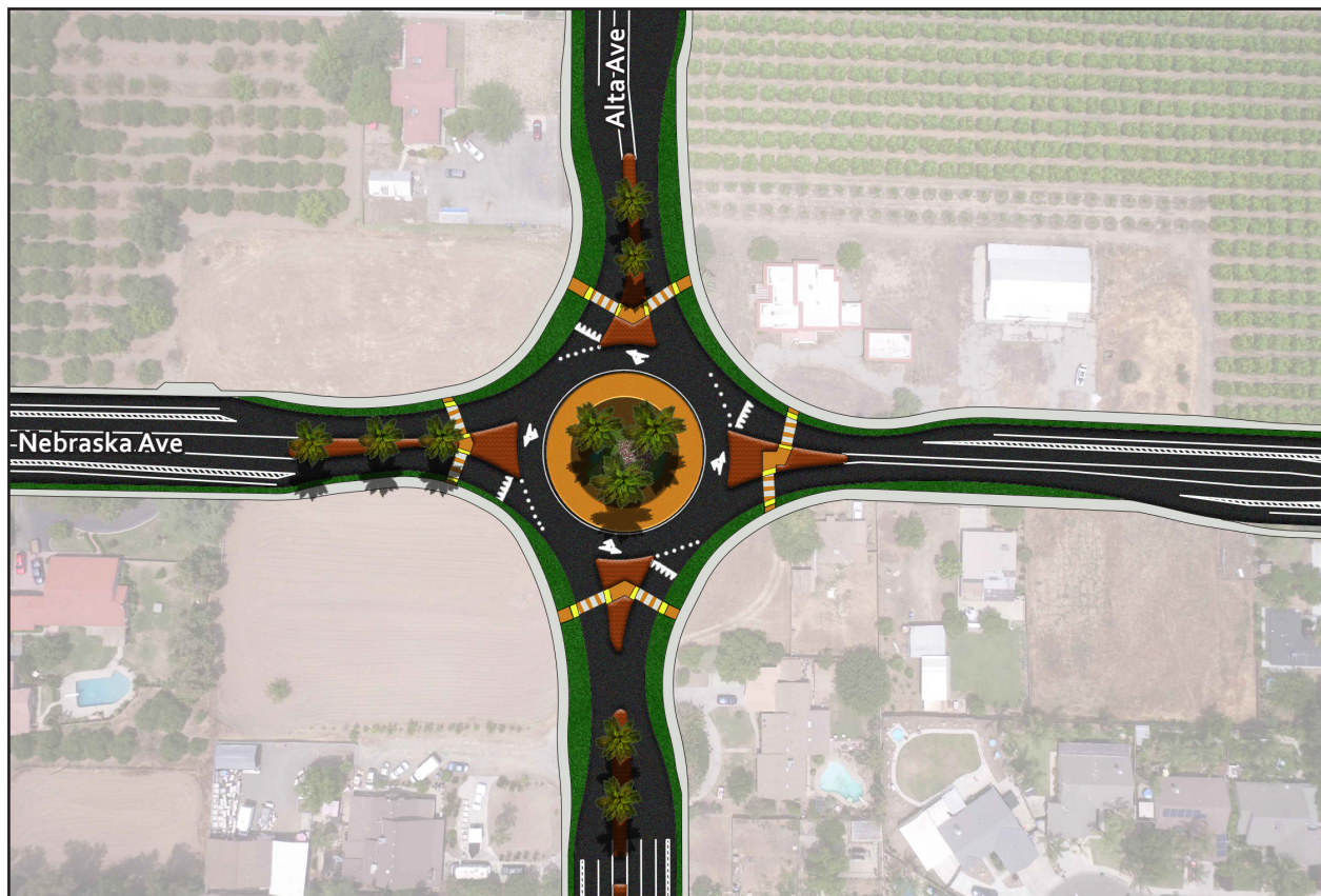
Figure 4-4. Proposed Design Concept for Alta Avenue & Nebraska Avenue
