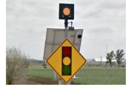
Advance warning signs (E:2, C:1, IC:1)
