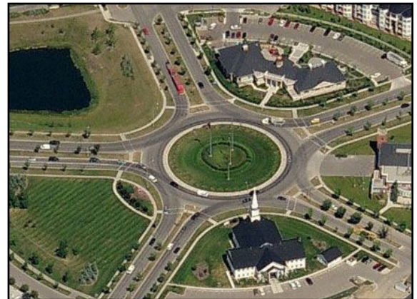
Figure 3-5. Example of rotary intersection.
