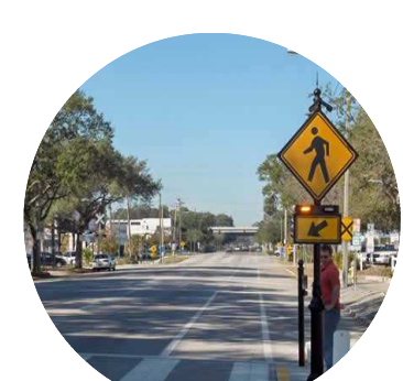
Rectangular Rapid Flashing Beacons
